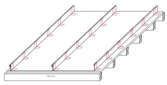
In all wind zones, it is Steelformers standard practice that the clips are to be fixed to all ribs of all purlin lines (or nog/girt lines for wall applications).
